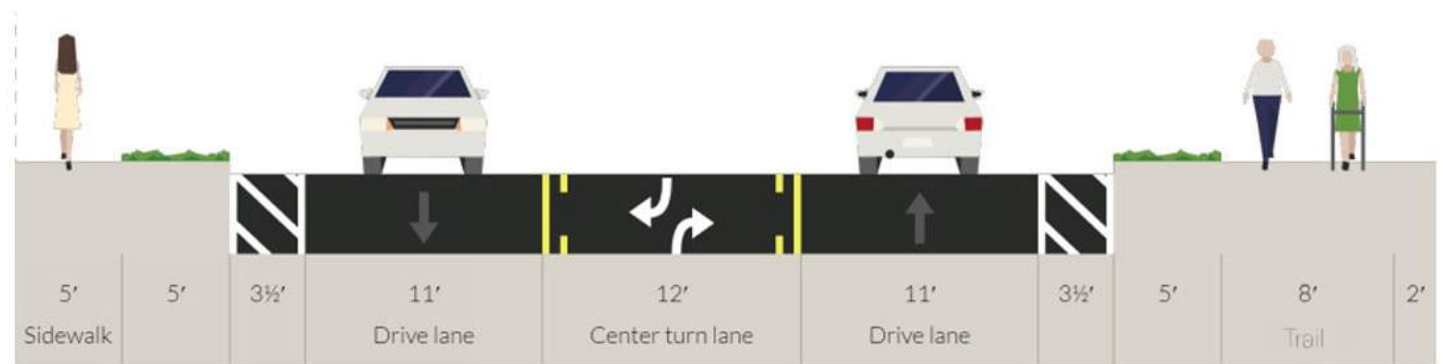
FIGURE 4. CSAH 6 (MISSISSIPPI STREET) TYPICAL SECTIONS
